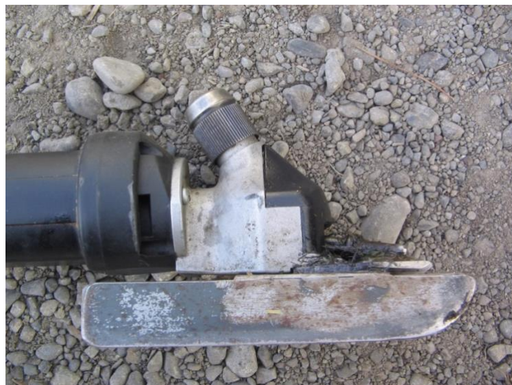
Figure 5: Shearing shears with a sled attachment to sample the pasture in the exclusion cages to a height of 25mm.
