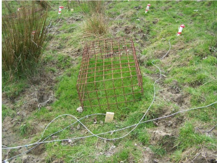
Figure 13: Pugging damage from cattle over the winter months at Site A, leading to a change in preferential flows for surface water, compaction of topsoil and overall reduction in pasture growth.
