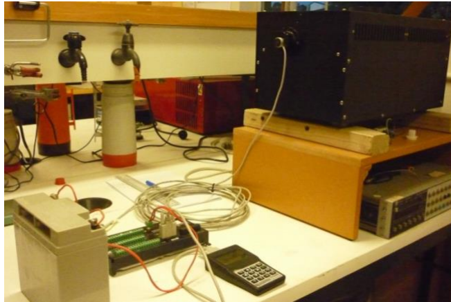
Figure 7: A reference standard light source (Li-Cor model 1800-01) was used to calibrate each of the quantum sensors prior to installation in the field experiment.
